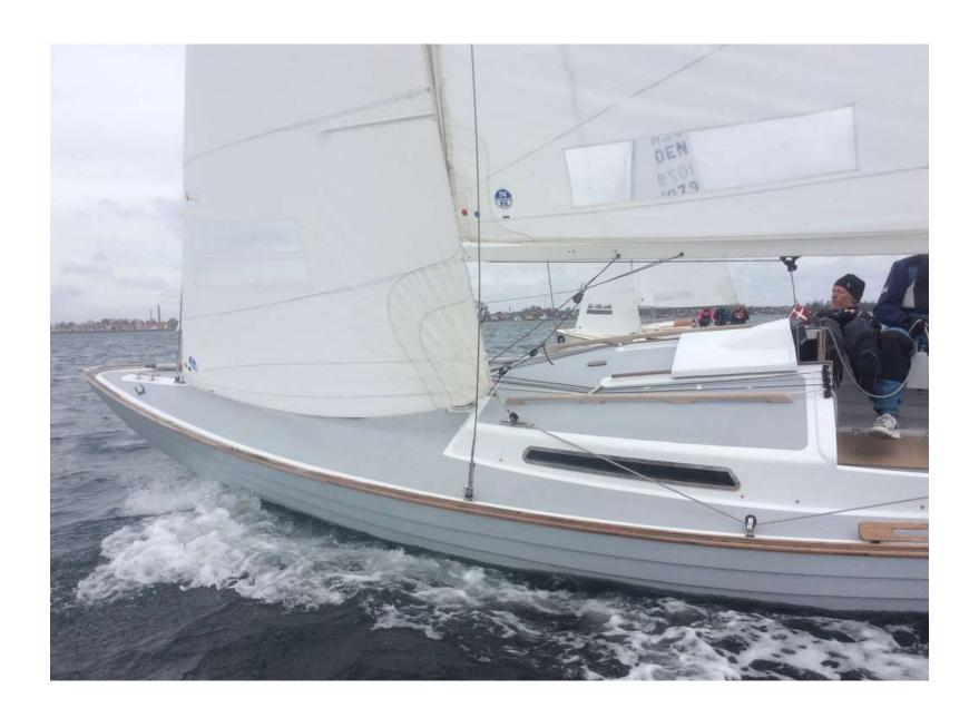
**2 Jib Sheet;** As a rule, sheet the jib so that the middle batten is parallel to the centerline in most conditions, but in light winds (0-5 knots) leave 2-3 degrees of twist. If the sea is lumpy, move the jib lead two to three "holes" forward to get more draft and power in the jib (the middle batten shall still be parallel to the boat's centerline). In heavy winds move the lead on to two "holes" back without letting the foot of the sail become loose and flutter.
