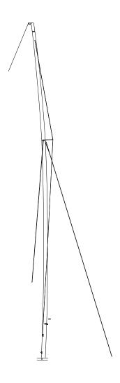
**Jumper struts;** legs not less than 450 mm +- 5 mm. The distance between the bearing points of jumper struts shall be 900 mm+- 10 mm. This is standard dimensions on J.M and B.M mast
