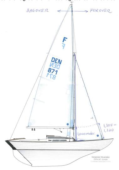
**3 Positioning the foot of the mast**. Move the foot of the mast aft until the mast just touches the aft edge of the mast hole in the deck. In light winds (0-8 knots) the mast should be relatively hard on the aft edge and pressed 22 mm astern on the mast foot rail, the mast will bend smoothly. In the wind range 9-14 knots of wind, press the foot of the mast 16 mm astern and in strong winds 10 mm astern.
