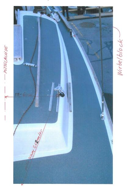
**1. Sheeting Point,** The position of the jib lead is crucial for the jib trim. As a reference point measure 2.65 m from the pin in the forestay to the centre of the block (if the lead is on the cabin top). The jib shall luff evenly, i.e. tell-tales must fly at the same time in top and bottom.
